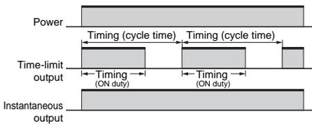
The Timer starts when the power comes ON or when the reset input goes OFF.
