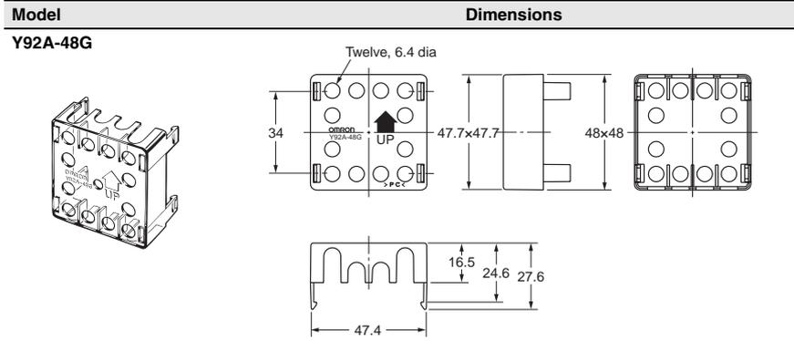
**Note:** The Terminal Cover can be used with a Back-mounting Socket (P3G-08 or P3GA-11) to create a finger-safe construction.
