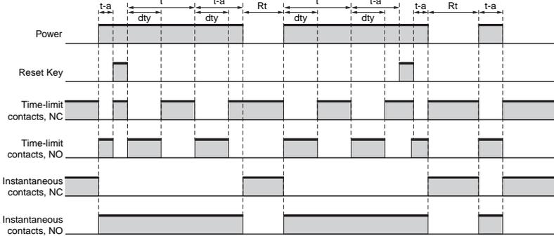
t = Set time, dty = ON duty time, Rt = Reset time (0.5 s min.), t - a < t (Indicates the time is less than the set time.)
