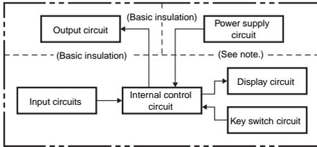
**Note:** Basic insulation is provided between the power supply circuit and the input circuits. However, basic insulation is not provided in the H5CX-□D-N.
