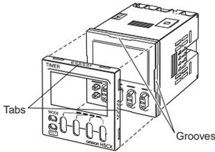
The Front Panel is attached to the Terminal with tabs in four locations. To remove the Front Panel, open the tabs and pull the Front Panel forward. To attach the Front Panel, press it onto the Timer so that all four tabs lodge into the grooves on the body of the Timer.
