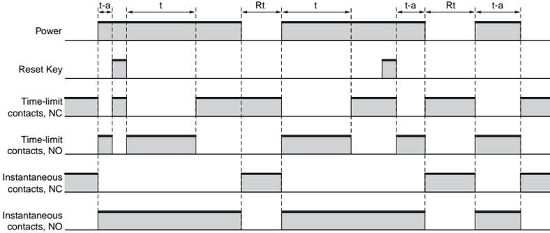
t = Set time, Rt = Reset time (0.5 s min.), t - a < t (Indicates the time is less than the set time.)
