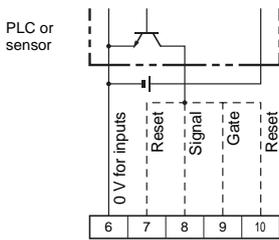
**Note:** Operate with transistor ON
