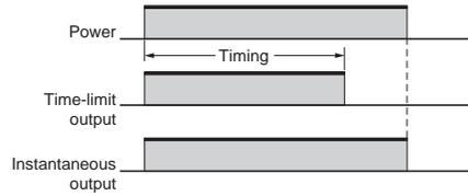
The Timer starts when the power comes ON or when the reset input goes OFF.
