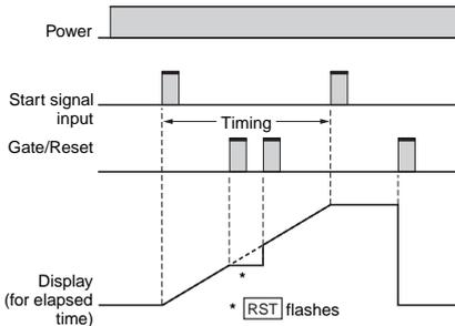
The signal starts and stops timing.
