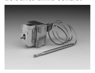
The LC Series Limit Control is designed for any appliance where protection from over temperature is needed. All LC Series controls are non-adjustable, factory calibrated, and feature negative based power element diaphragms.
