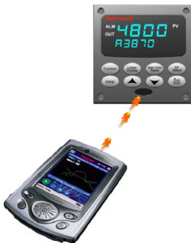
Figure 1-3 Depiction of infrared communications
