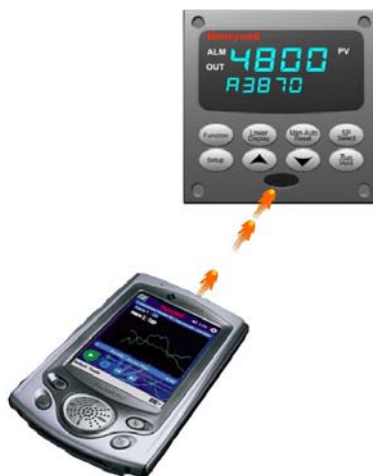
Figure 1-3 Depiction of infrared communications
