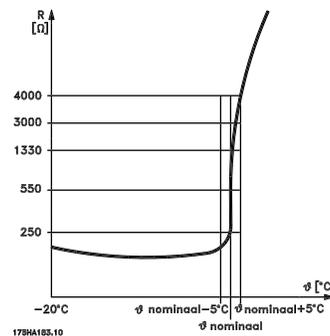
If a motor features a Klaxon thermal switch instead, this can also be connected to the input. If motors operate in parallel, the thermistors/thermal switches can be connected in series (total resistance lower than 3 kΩ). Parameter 128 *Motor thermal protection* must be programmed for *Thermistor warning* [1] or *Thermistor trip* [2], and the thermistor is to be connected between a digital input and terminal 50 (+10 V supply).
