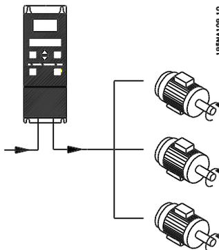
The adjustable frequency drive is able to control several motors connected in parallel. If the motors are to have different rpm values, use motors with different rated rpm values. Motor rpm is changed simultaneously, which means that the ratio between the rated rpm values is maintained across the range. The total current consumption of the motors is not to exceed the maximum rated output current  $I_{INV}$  for the adjustable frequency drive.
