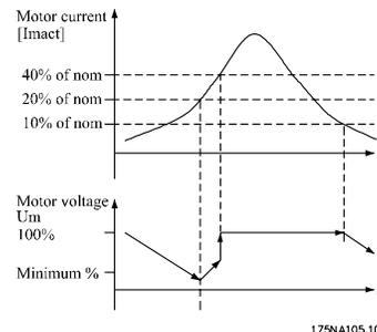
If the active motor current is below 10%, the motor voltage will be decreased by the speed mentioned above until the voltage reaches the setting for Par. 117. If the active motor current comes over 20% the voltage will be increased by the above-mentioned speed. If the active motor current reaches 40% the motor voltage will be increased immediately to normal motor voltage.
