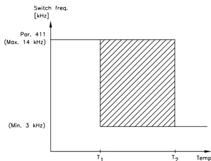
When using the LC filter the minimum switch frequency is 4.5 kHz.
