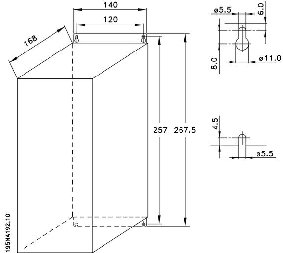
The drawing below gives the mechanical dimensions of VLT 2822 (3 HP) 200-240 Volts and VLT 2822-2840 (3 - 5 HP) 380-480 Volts. All dimensions are in inches.
