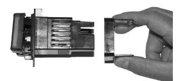
3. For an IP66/NEMA 4X seal, place the blade of a screw driver in the notch of the mounting collar assembly and push to ward the panel while applying pressure to the face of the RUI. Don't be afraid to apply enough pressure to properly install the RUI. If you can move the case assembly back and forth in the cutout, you do not have a proper seal.
