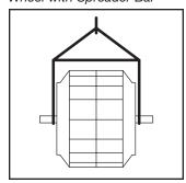
not support the shaft or the wheel on housing sides. Use only the key provided with the shaft and wheel.
