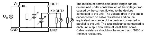
Electrical diagram for current outputs
