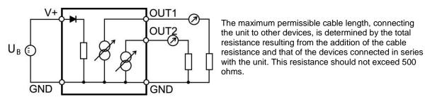
Terminal block diagram (analog outputs only)
