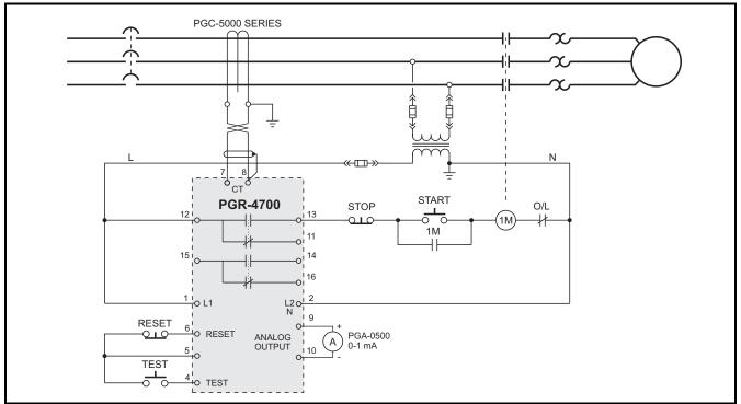
FIGURE 2. Typical Connection Diagram.
