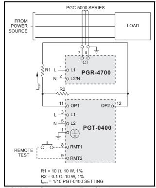
FIGURE 7. Ground-Fault-Test Circuit.
