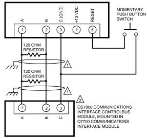
THREE WIRE SHIELDED CABLE MAY BE REQUIRED. TWO 120 OHM TERMINATING RESISTORS ARE REQUIRED FOR CONNECTIONS OVER 100 FEET (30 METERS). CABLE SHIELD MUST BE TERMINATED TO EARTH GROUND AT BOTH ENDS. IF SHIELDED CABLE IS NOT USED, TWISTED PAIR WIRE MUST BE USED.
