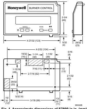
Fig. 1. Approximate dimensions of S7800 in in. (mm).
