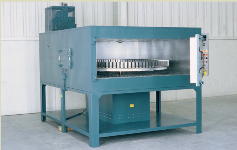
This Rotary Hearth oven provides preheated gears... ready on demand, one at a time.
