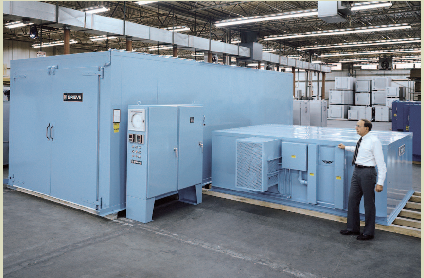
This Walk-in Oven, with its top-mounted air heater removed for shipment, gets one final look.
