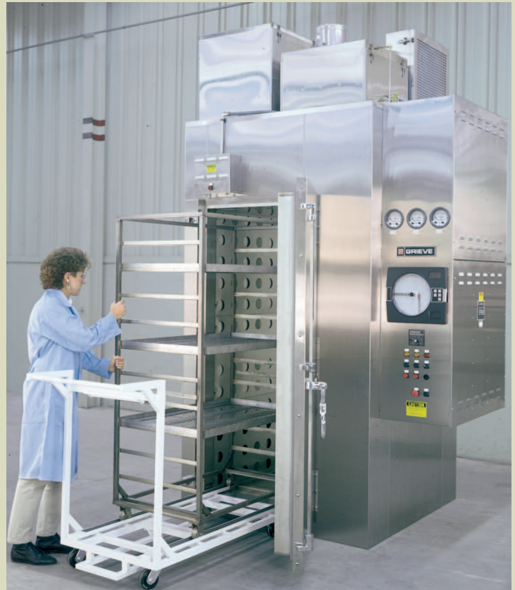
This Class 100 Sterilization Oven is used for the depyrogenation of glass, teflon, and other heat resistant materials. It features a stainless steel shelf truck, as well as an exterior truck transfer dolly.
