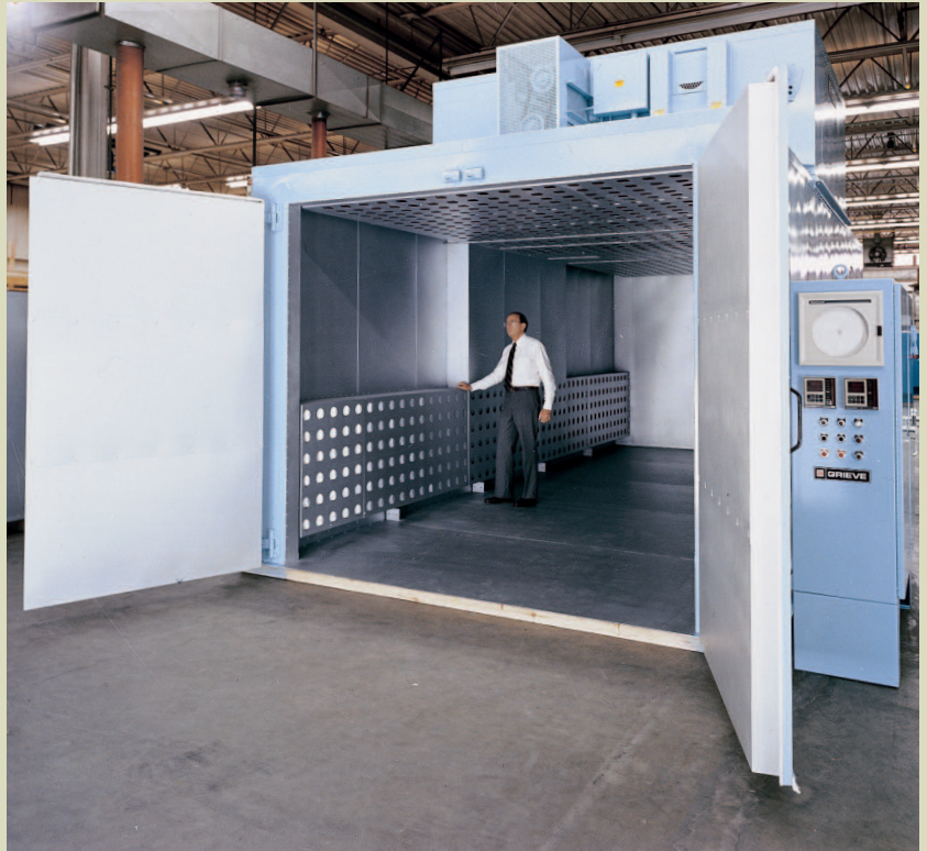
A 9' wide x 24' deep x 8' high batch oven for curing large loads of rubber parts. It features a removable top-mounted heat chamber and free standing control panel.
