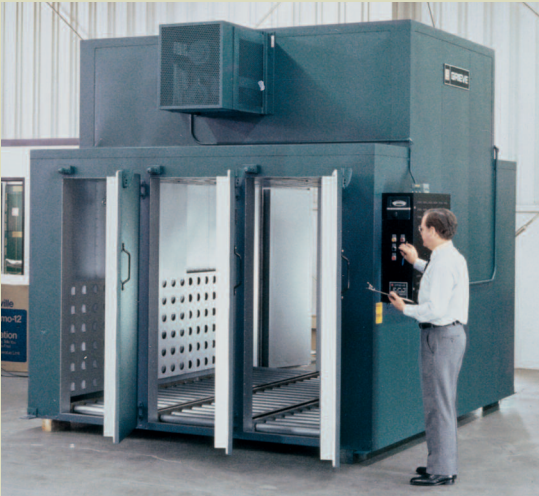
This Walk-In unit features multiple access doors at each end, plus three individual roller lanes designed to accommodate the customer's loading requirements.
