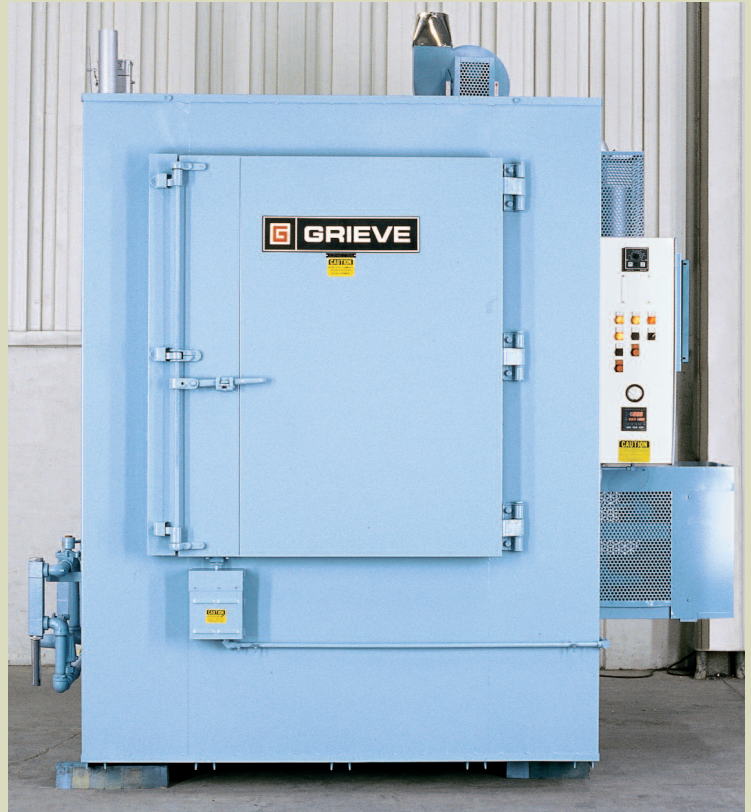
A 750°C Inert Atmosphere Oven, for processing specialty ceramic parts, includes air quench as well as cooling by jacketed interior.
