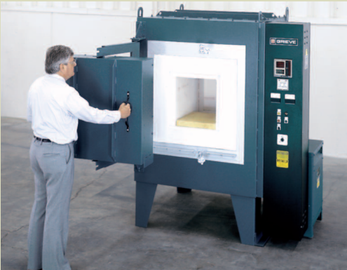
The massive door on this high temperature furnace is checked for proper balance and fit.
