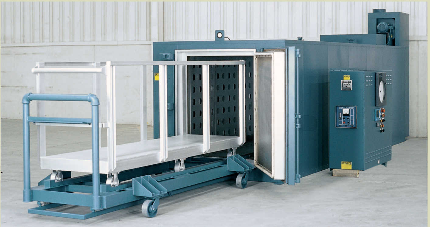
Truck and dolly loading allows annealing bundles of plastic rods in an inert atmosphere.
