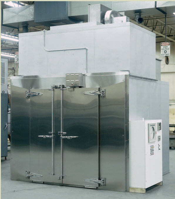
A 500°F Electrically-Heated Sterilizing Oven for sterilizing large loads of glassware. It features double doors at each end of the oven for "pass through" operation. Removable top mounted heat chamber, sealing flange and remote control panel aided in installation between customer's wash area and clean room.
