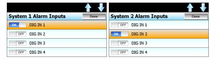
For example, if digital input 1 will be used for the system 1 failure input, then select digital input 1 from the list. If digital input 2 will be used for the system 2 failure input, select it as the alarm input for system 2. Additional inputs can be selected if necessary. Once all selections have been made, press the 'Done' button to accept the input selections and return to the Redundancy Setup screen.
