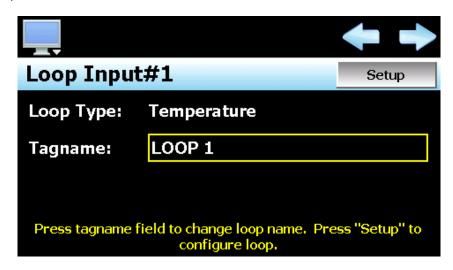
The left and right scroll (arrow) buttons allow the user access each loop in the system, by pressing left or right to go to the previous or next loop.
