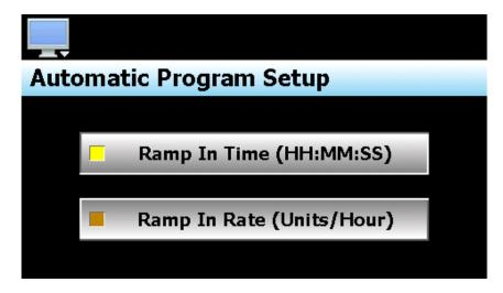
When **Ramp In Time** is selected, the steps of the automatic program are entered as units of time in hours, minutes and seconds with individual set points for each control loop in the system. When the steps of the program are executed, the programmer will ramp the set points of each loop individually to the set point of the step, linearly over the time duration of the step.
