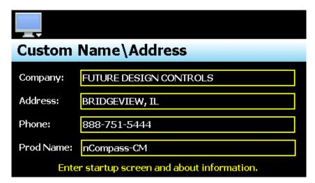
To edit the company, address, phone number or controller (product) name, press the field and enter the desired text. Each field can be entered with a maximum of 24 characters that will be displayed on the splash screen when nCompass starts.
