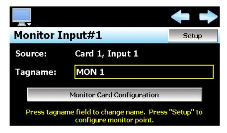
The left and right scroll (arrow) buttons allow the user access each monitor point in the system, by pressing left or right to go to the previous or next monitor point.
