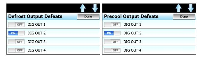
For example, if digital output 2 is used as the control output for the system fans when a system event is turned on, then select digital output 2 from the list. This will turn off the fans during defrost and precool whenever the defrost cycle is active. Additional outputs can be selected if necessary. Once all selections have been made, press the 'Done' button to accept the defeat selections and return to the Defrost Setup screen.
