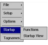
The **Startup** menu provides access to enable and disable nCompass runtime screens/menus and the select the desired startup view.
