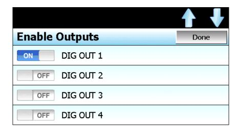
For example, if digital output 1 is used as a control output to turn on a circulating fans that are common to both system 1 and system 2 when a system event is turned on, then select digital output 1 from the list. This will enable the redundancy logic whenever the circulating fans are on. Additional outputs can be selected if necessary. Once all selections have been made, press the 'Done' button to accept the output selections and return to the Redundancy Setup screen.
