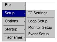
The **Setup** menu provides access to the primary controller setup options. These options include the number of loops and monitors used, the number of digital and analog inputs and outputs available, the number of alarms and events available as well as loop, monitor and event configuration.
