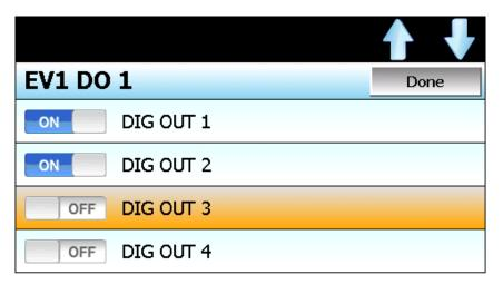
Select each output that is to be assigned to the event from the list and press the 'Done' button to assign the outputs to the event and return to the Event Setup screen.
