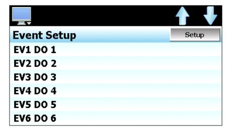
To assign outputs to an event, touch the desired event in the list box to select it and press the 'Setup' button. The 'System Event Output Configuration' screen will then be shown.
