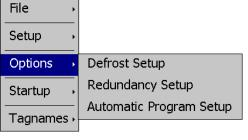
The **Options** menu provides access to additional controller options including the setup of defrost and redundancy operation as well as the automatic programmer mode of operation.
