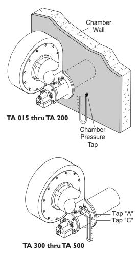
Step 3a: Ignite the burner (Option I: Burner not equipped with bypass start gas)
