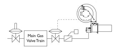
Step 3b: Ignite the burner (Option 2: Burner equipped with bypass start gas) I. Drive the gas control valve to low fire.
