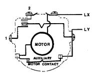
The AB4 has a single poie, double throw switch and a motor cut-out switch. Load switch contacts LY and 1 are normally closed. When pointer is turned to any point on timing scale, contacts LY and 1 open and LY and 2 close. Auxiliary motor contacts also close and start timing motor. When pointer is at 0 (timed out), only LY and 1 are closed. When pointer is turned to "Hold", contacts LY and 1 open and LY and 2 close without starting the timer motor.
