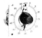
The MANUFLEX® AB Series timer is a manually set, synchronous motor driven timer, adjustable to a selected time range by a large, easy to read set pointer. To operate, turn the set pointer to the required time interval. A load circuit is closed when the pointer is turned from zero. The timer motor drives the pointer back to zero, at which point the load circuit opens. Timer is used where a device is to be turned on, runs a selected time and stops at the end of the time interval.
