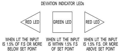
On Time Proportioning and Proportional models if the input stabilizes below the set point then the Offset Correct adjustment should be turned clockwise in small increments until the deviation indicator green LED is lit. If the input stabilizes above the set point then adjust the Offset Correct counterclockwise.
