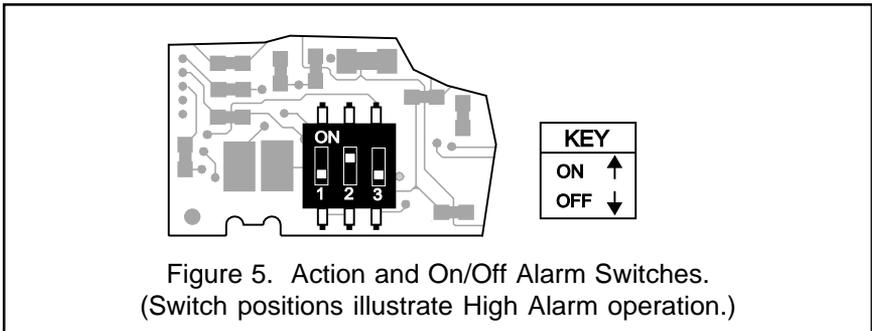
For newer models select the action by setting switch 1 on and switch 2 off (direct acting) or switch 1 off and switch 2 on (reverse acting). Switch 3 determines whether the output will reset after the temperature has moved to the other side of the set point. If switch 3 is on then the output will automatically reset. If switch 3 is off then the RESET button on the front of the control must be pushed before the output will reset.
