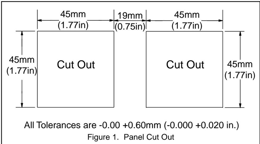
From the front of the panel, slide the housing through the cut out. The housing gasket should be against the housing flange before installing. From the rear of the panel slide the mounting collar over the housing. Hold the housing with one hand and using the other hand, push the collar evenly against the panel until the spring loops are slightly compressed. The ratchets will hold the mounting collar and housing in place.
