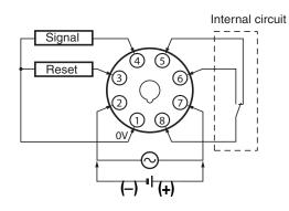
The power supply and input circuit are not insulated. Terminals one and two of the 700-HX are connected internally.
