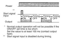
Sustained Output Powe Start signal Reset Control output OFF time UP ON time Timing diagram OFF time DOWN ON time 0
