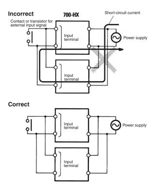
It is impossible to provide two independent power switches as shown below regardless of whether or not the timers are different in phase.
