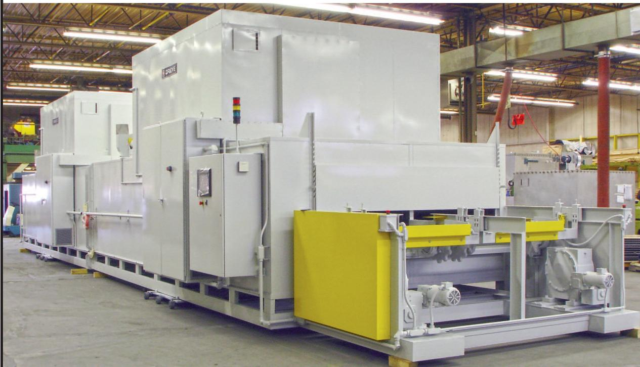
**TWO ZONE, DUAL BELT CONVEYOR OVEN, Serial No. 95859A1108**
